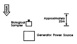
Figure 5-15c. Correct Placement of Sampler With A Generator Power Source.
